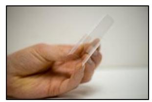
According to Susan Hirst, Product Development Manager for Abrisa Technologies, SCHOTT D 263® T eco ultra-thin glass can be custom fabricated to meet individual customer specifications. It is an excellent choice for ultra-lightweight mobility and scanning applications, ultra-low-profile displays and devices, miniature and micro-electronics and sensors and chemical process resistant slides and sample platforms."
