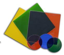
Dichroic and color correction filters have the advantage of reflecting unwanted light instead of absorbing the energy, which allows dichroic filters to be used with much higher intensity light sources up to 550°F.
